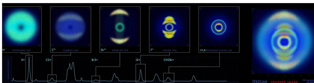
Figure 3. 2D image for each mass ion with TOF information can be reconstructed in any time window.
