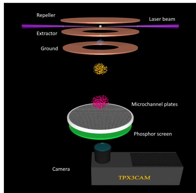
Figure 2. Typical velocity map imaging setup. The VMI setup normally consists of electrostatic lenses, microchannel plates (MCPs), phosphor screen, e.g. P46, P47, etc., and an optical camera. Here the CCD camera has been replaced by a TPX3CAM detector.
