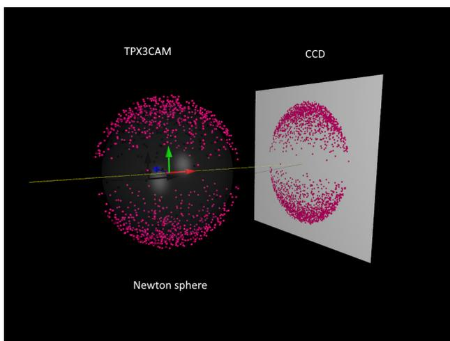
Figure 1. Newton Sphere of ion fragments generated in photofragmentation. A CCD camera records 2D integral images of the Newton Sphere. Replacing the CCD camera with ASI TPX3CAM, one can record event list (X, Y, TOF) for all ions and thus do a direct measurement of the Newton Sphere
